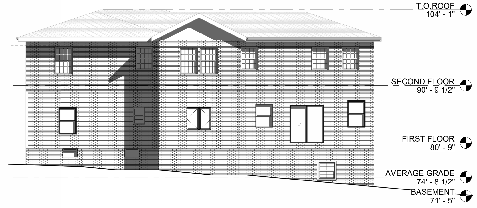
3 ELEVATION - EXISTING REAR ELEVATION 1/8" = 1'-0"
