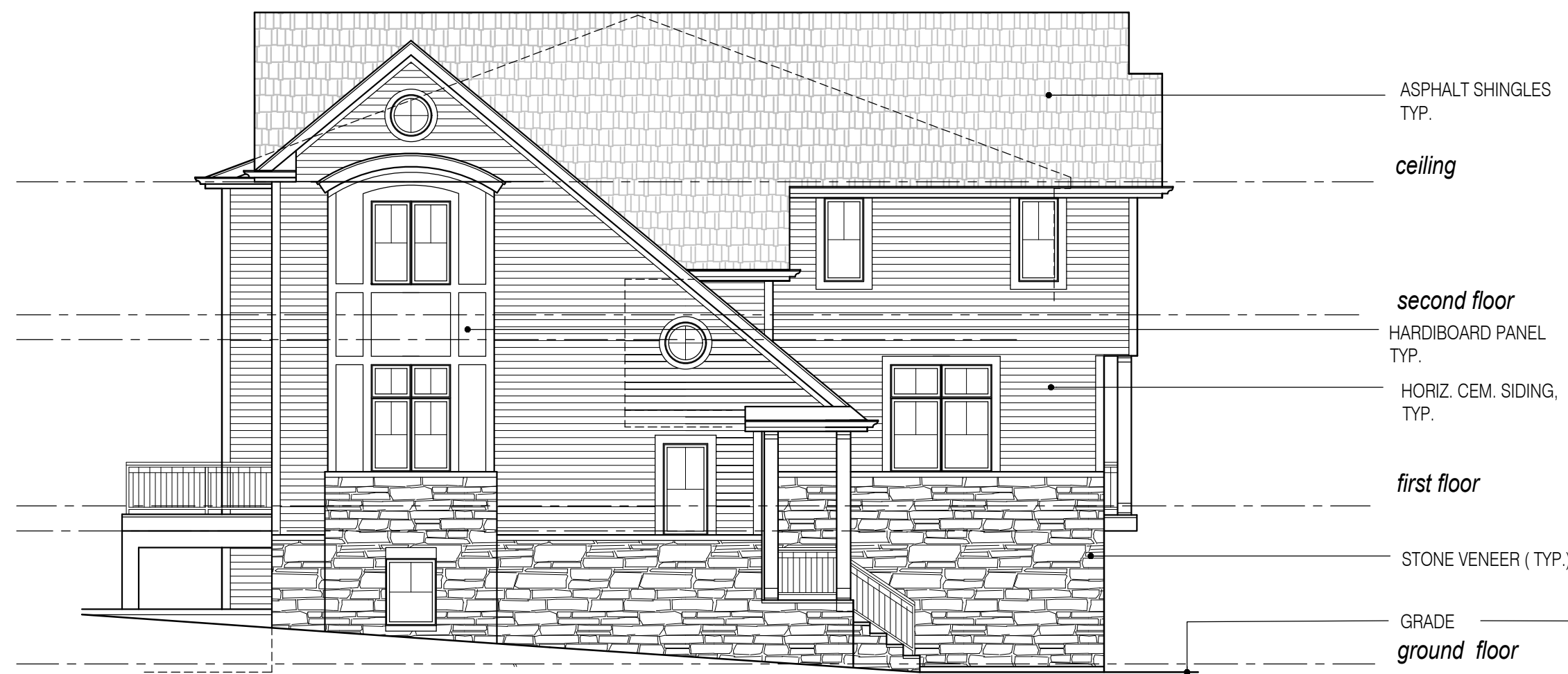
Left Side (Hardenburgh Road) Elevation - Building 1 1/8" = 1'-0"
