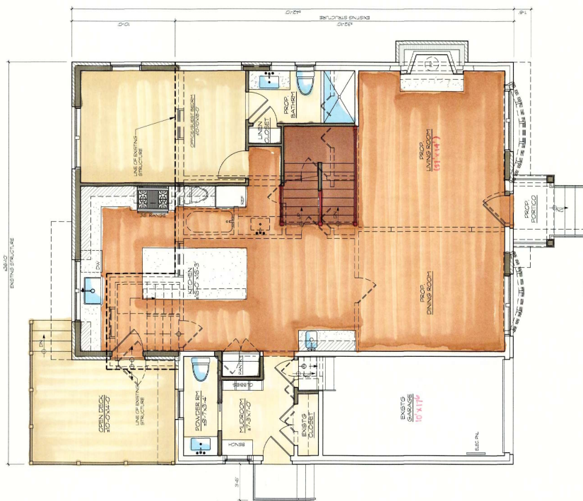
1 PROPOSED FIRST FLOOR PLAN SCALE 1/4" = 1'-0" EXISTING LIVABLE AREA 1,556 SQFT PROPOSED LIVABLE AREA 1,577 SQFT GARAGE 1,077 SQFT
